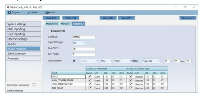
Expander *iO* has: terminals for 1 input, 1 output (relay contacts) and 1-Wire serial bus for connecting temperature sensors. Relay output can be controlled according to logical (AND, OR, XOR) conditions.
