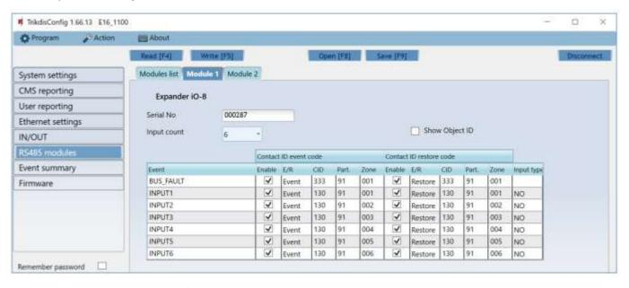
Expander iO-8 has 8 universal (input/output) terminal contacts. Up to four iO-8 expanders can be connected.
