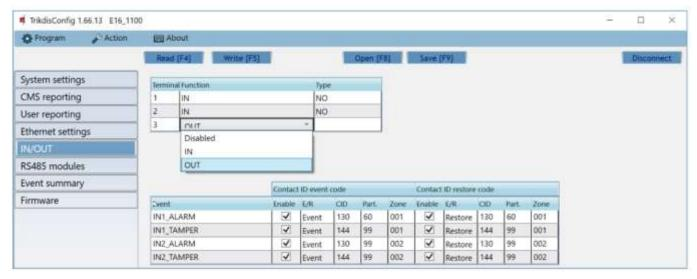
The communicator has 3 universal (input / output) terminals. The table can set the terminal operating mode (Off, IN, OUT). The input must specify the type of circuit to be connected NC, NO, NO / EOL, NC / EOL, NO / DEOL, NC / DEOL.
