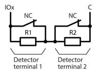
Normaly closed with EOL, with tamper and wire fault recognition (ATZ\_T)
